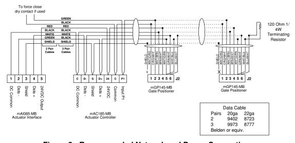
Figure 3 - Recommended Network and Power Connections
